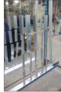
Figure 2 – Hooked parts to start anodizing process
